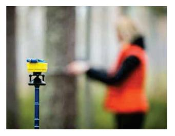
The yellow T3 transponder is used for ultrasound measurements with the Vertex IV. From February 2015, T3 transponders for the ultrasound function in VL5 instruments will be delivered in a bright orange color.
