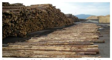
Start in one corner of the pile. Measure pile length and several heights for an average pile height. Divide pile in sections if needed. State width (log length), assortment, wood volume factor, and height for each section.
