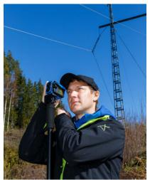
The Laser Geo is a great investment to improve efficiency for different measuring jobs. Measure in open terrain and for distance measuring from 46cm up to 700 m. Use to measure tree heights and canopy, to map areas and trails, to measure terrain slopes, to store and process collected data. The Laser Geo includes built-in GPS and compass, it can be custom programmed, updated, and upgraded.
