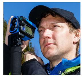
The Laser Geo 3D Pile allows you to estimate volume of irregular objects, such as a woodchip piles. Use a non-magnetic monopod for increased stability. Results are presented on large external graphic display and internal heads-up display. Measure, process, store, transfer - all in one compact unit.
